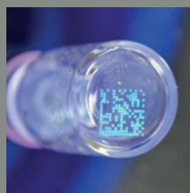
V459-D UV ink on glass vial bottom
